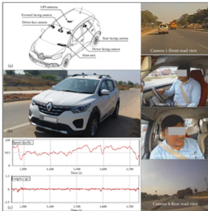
Figure 13: (a) Instrumentation details; (b) Study vehicle; (c) Recorded speed and acceleration profiles; and snapshots of collected video data.
